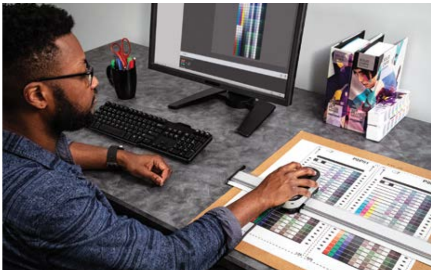
i1Publish Pro 3 assists in the formation of custom profiles for RGB, CMYK and CMYK+4 printers
