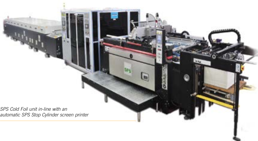
Cold Foil is applied by two rubberised rollers on top of a large size diameter cylinder drum
