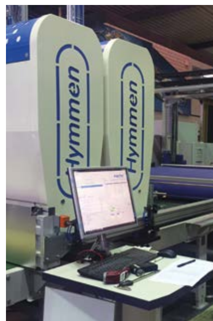
Figure 10: The JUPITER Digital Printing Line for DLE here with two rows of printing heads at the Hymmen technology centre
