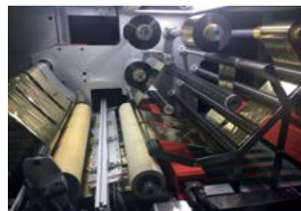
Cold Foil is applied by two rubberised rollers on top of a large size diameter cylinder drum
