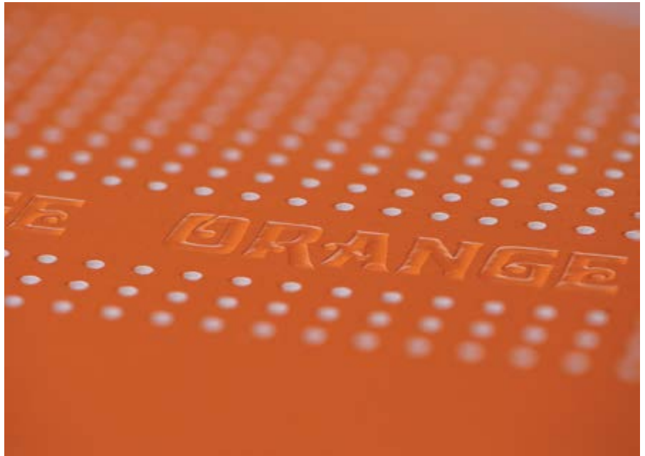
Partial clear varnish with SEFAR PET 1500 165/420-34Y TW (UV inks) or SEFAR PET 1500 77/195-55Y PW (solvent inks)
