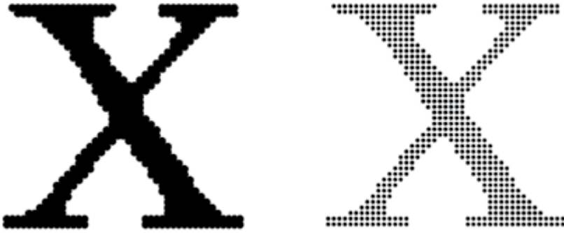
Figure 6: The effect of dot size on colour density
