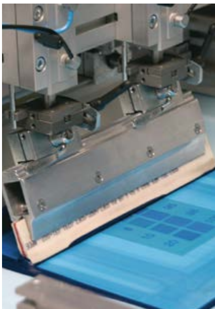
Adhesive printed through a stencil with a squeegee
