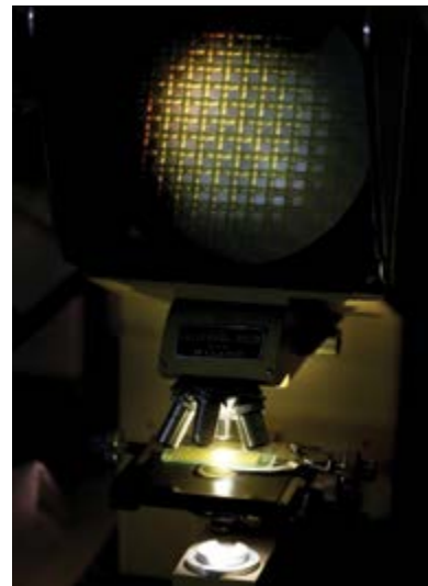
Extris screen fabrics mesh details 125X (magnification)
