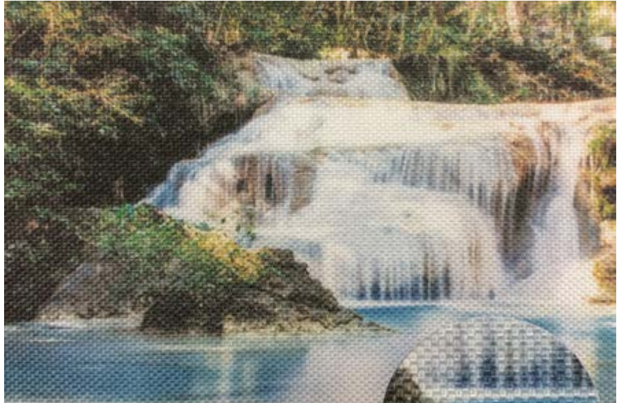
This piece of Cordova nylon fabric was pre-treated using a polyester CMYK pre-treat fluid and printed with Brother GT-3 inks. (Image courtesy Brother International Corporation)
