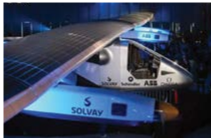
Screen-printed photovoltaic panels on record flight: "Solar Impulse 2" around the world with no fuel
