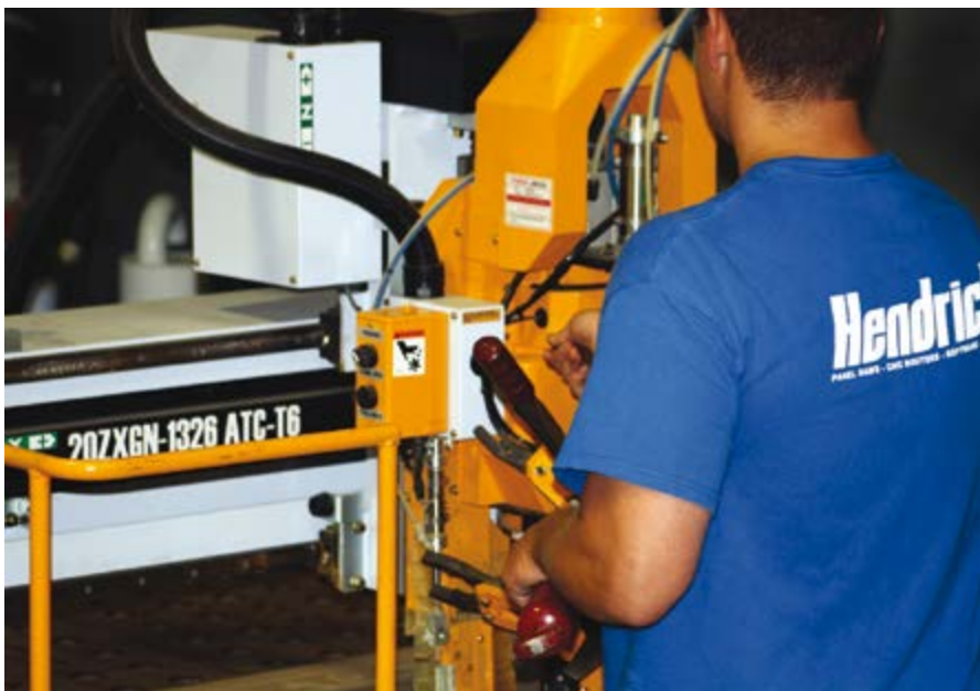
Semi-annual router spindle lubrication on Hendrick 20ZXGN CNC router
