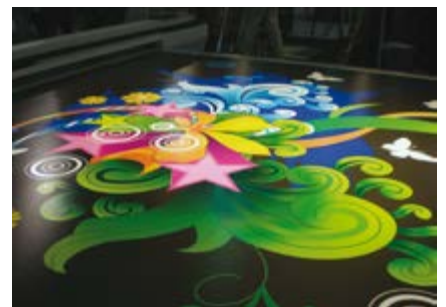
This example of white ink in an opaque application shows where white forms part of the image content, and creates a base for the CMYK colour set.
