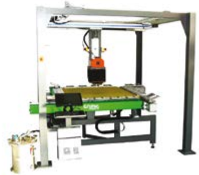
G-BOND ULTRA CURE Automatic stretching machine with UV-gluing robot
