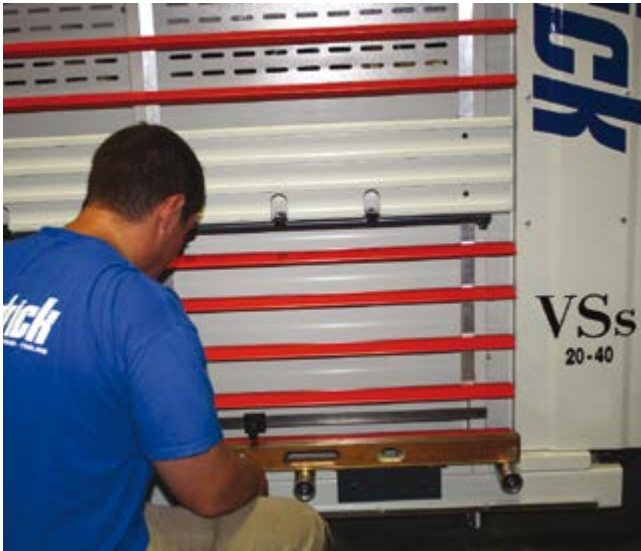
Monthly inspection of material support rollers for Hendrick VSs vertical panel saw
