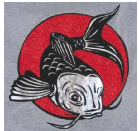
This special effect 'best' koi design utilises Cad-Cut Hologram (mirror), black MultiFlock and red Glitterflake.
