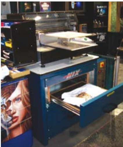
A Brother 541 digital garment printer mounted on top of the HIX two drawer Verticure digital garment dryer
