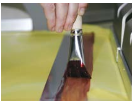
Application of screen adhesive
