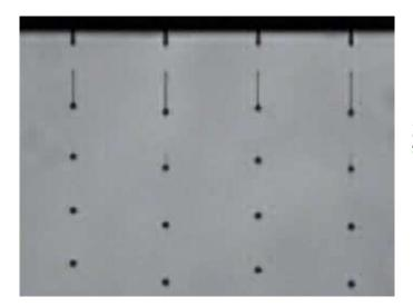
Ink exiting the nozzle array of a piezo print head other components. Some of these materials can have properties which produce foams or can entrap air.
