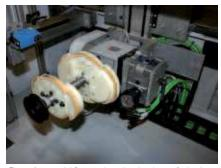
Figure 4: a special fixture adapted to the shape of a bucket ensures repeatable hold
