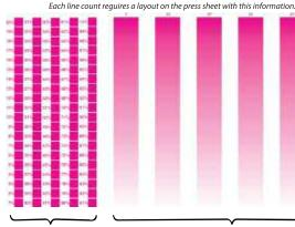
This is the 100 Step test to determine the correct film curve Figure 3: LPI and angle test
