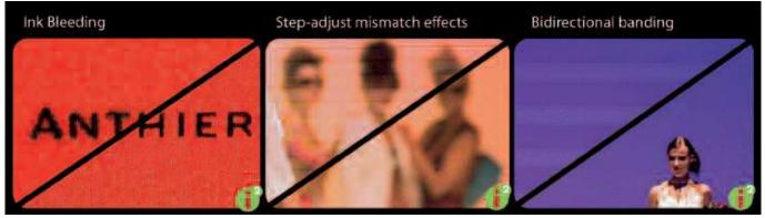
Figure 1: common line printing problems
