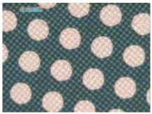
Sefar PET 1500 120-34 Y mesh – diameter of the dots is approximately 165µm
