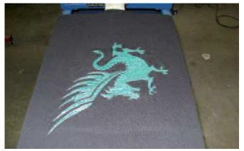
Figure 5: The printed image shows the ridges and creases left behind
