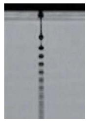
Satellites are smaller than normal droplets and land on the substrate in random positions
