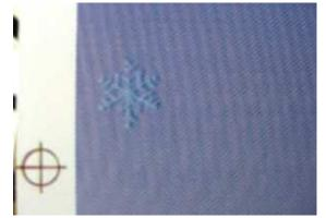
Every mesh count has only a very few line counts (2 to 3) that are compatible with the mesh. Compatible means there are at least three angles 30 degrees apart that are realitively moire free. Figure 2: Mesh count versus LPI moiré
