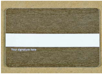
Signature field printed with NoriCure CCI UV ink
