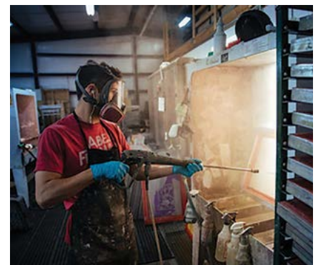
A typical way to wash out screens. Photo: Printed Threads
