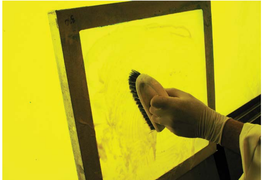
Reclaiming and degreasing a screen
