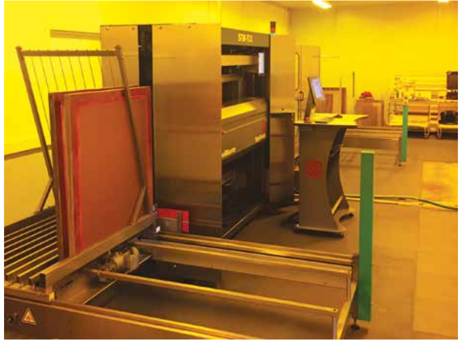
SignTronic STM TEX Pro 10online unit at Decordecad. For a perfect screen lab SignTronic recommends yellow light (UV-free light conditions)
