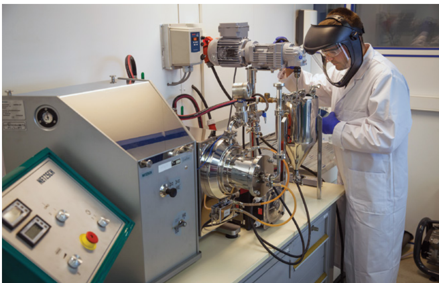
Figure 5: Preparation of an inkjet grade nanodispersion in a bead mill using tailor-made dispersing agents
