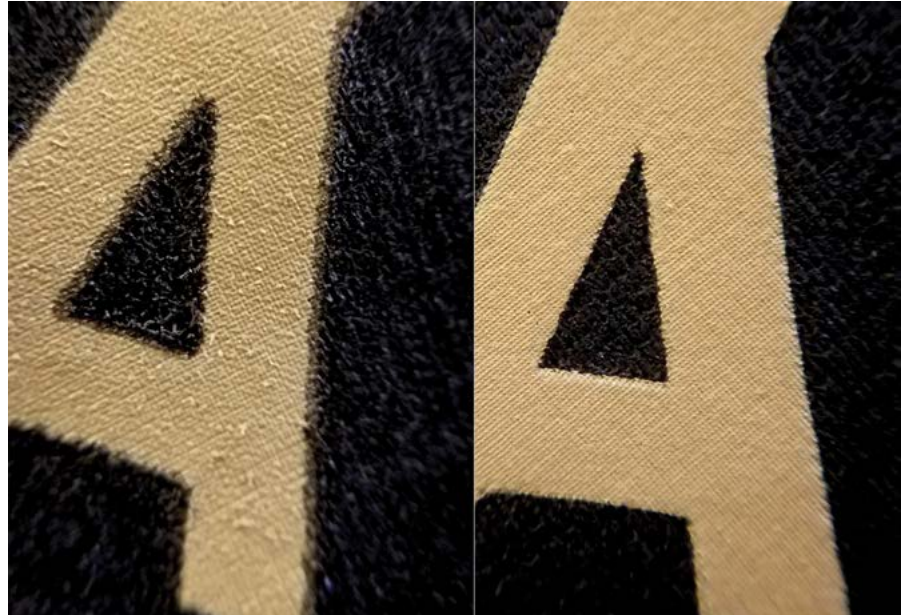
Invest in better quality equipment. Example printed with loose mesh (left). Edges are much more crisp and defined when printed with tight mesh (right)
